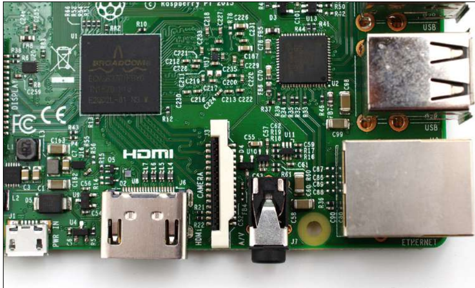
FIGURE 15-2: The Raspberry Pi's CSI connector, pictured on a Raspberry Pi 3 Model B
