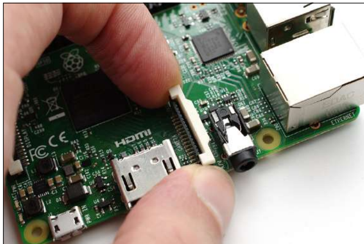
FIGURE 15-3: Raising the lugs of the CSI connector prior to inserting the ribbon cable
